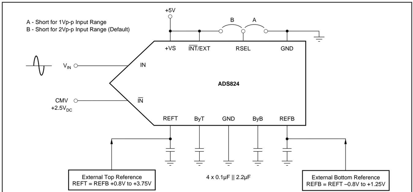
FIGURE 8. Configuration Example for External Reference Operation.
