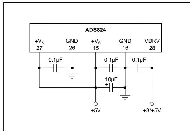
FIGURE 9. Recommended Bypassing for the Supply Pins.
