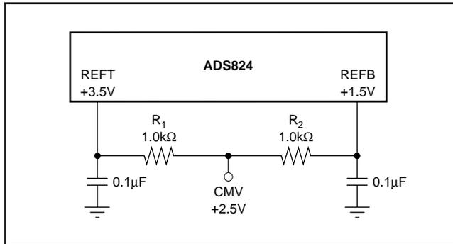
FIGURE 7. Alternative Circuit to Generate CM Voltage.
