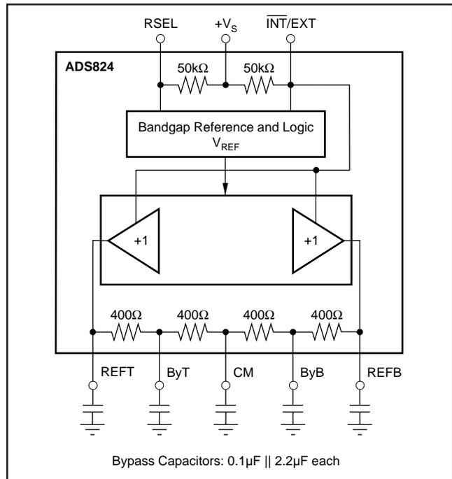
FIGURE 6. Equivalent Reference Circuit with Recommended
