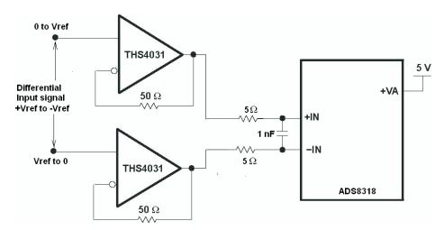
Figure 58. Unipolar Differential Input Drive Configuration
