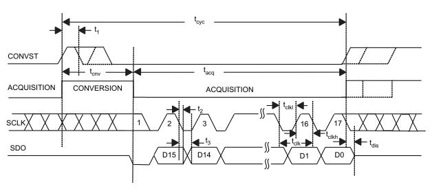
Figure 48. Interface Timing Diagram, 3 Wire CS Mode With Busy Indicator (SDI = 1)
