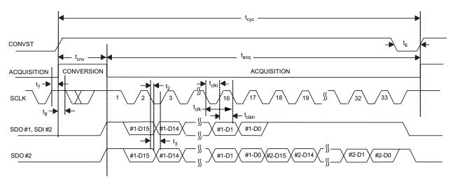
Figure 56. Interface Timing Diagram, Daisy Chain Mode With Busy Indicator
