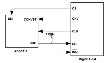
Figure 51. Connection Diagram, 4 Wire CS Mode With Busy Indicator
