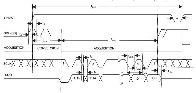
Figure 52. Interface Timing Diagram, 4 Wire CS Mode With Busy Indicator
