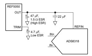
Figure 61. Direct External Reference Driving Circuit
