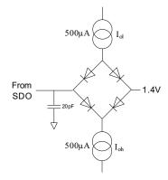
Figure 1. Load Circuit for Digital Interface Timing
