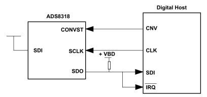
Figure 47. Connection Diagram, 3 Wire CS Mode With Busy Indicator
