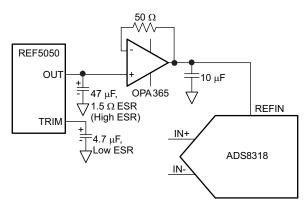
Figure 60. External Reference Driving Circuit
