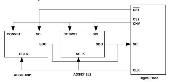
Figure 49. Connection Diagram, 4 Wire CS Mode Without Busy Indicator
