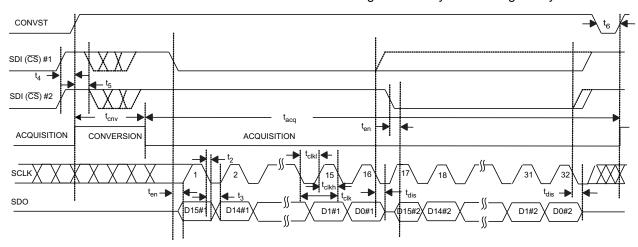
Figure 50. Interface Timing Diagram, 4 Wire CS Mode Without Busy Indicator
