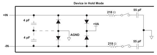
Figure 57. Input Equivalent Circuit
