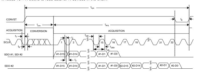
Figure 54. Interface Timing Diagram, Daisy Chain Mode Without Busy Indicator
