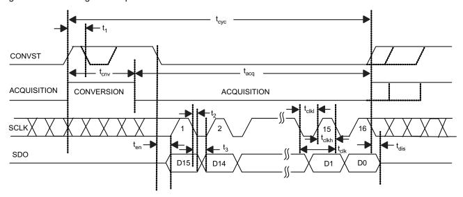
Figure 46. Interface Timing Diagram, 3 Wire CS Mode Without Busy Indicator (SDI = 1)
