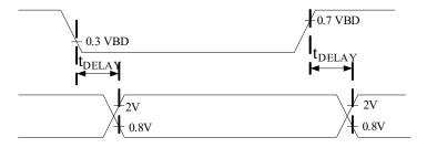
Figure 2. Voltage Levels for Timing
