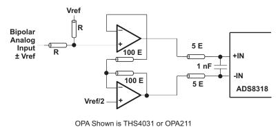
Figure 59. Bipolar Single-Ended Input Drive Configuration
