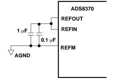
Figure 48. ADS8370 Using Internal Reference
