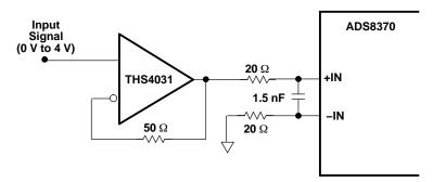
Figure 51. Unipolar Input Drive Configuration
