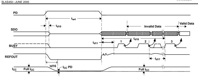
Figure 53. Device Full Power Down/Resume (Internal Refernce Used)
