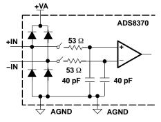
Figure 50. Simplified Analog Input
