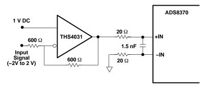
Figure 52. Bipolar Input Drive Configuration
