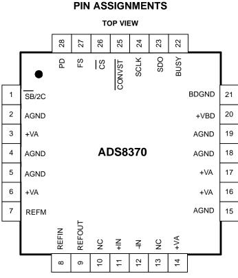
Note: The package thermal pad must be soldered to the printed circuit board for thermal and mechanical performance.
