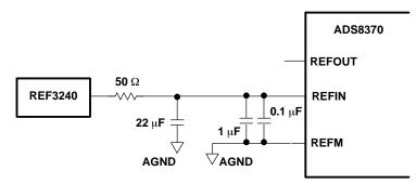
Figure 49. ADS8370 Using External Reference
