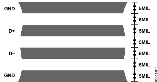
Figure 23. Typical Arrangement of Signal Tracks
