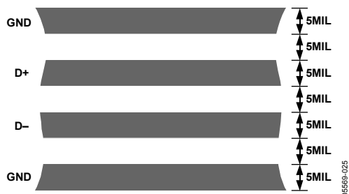
Figure 35. Typical Arrangement of Signal Tracks
