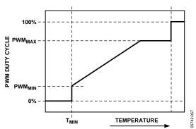
Figure 56. PWM<sub>MAX</sub> Determines Maximum PWM Duty Cycle Below the THERM Temperature Limit
