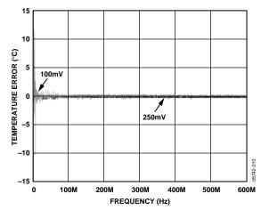
Figure 9. Internal Temperature Error vs. Power Supply Noise Frequency
