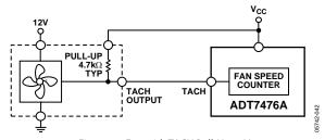
Figure 41. Fan with TACH Pull-Up to  $V_{\text{CC}}$
