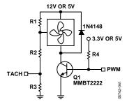
Figure 40. Planning for 3-Wire Fans on a PCB
