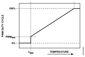
Figure 54. PWM<sub>MIN</sub> Determines Minimum PWM Duty Cycle
