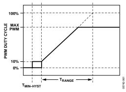
Figure 60. Changing PWM Max Does Not Change the AFC Slope
