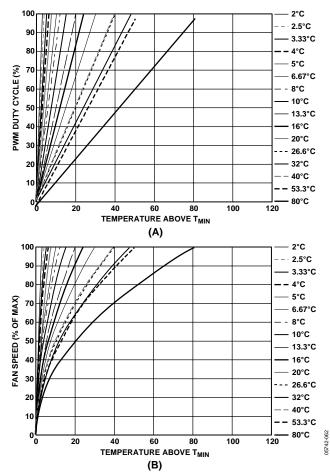
Figure 61. T<sub>RANGE</sub> vs. Actual Fan Speed (Not PWM Drive) Profile
