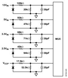
Figure 24. Structure of Analog Inputs
