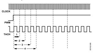
Figure 45. Fan Speed Measurement
