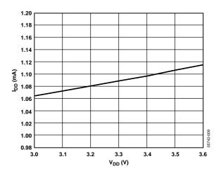
Figure 8. Normal IDD vs. Power Supply
