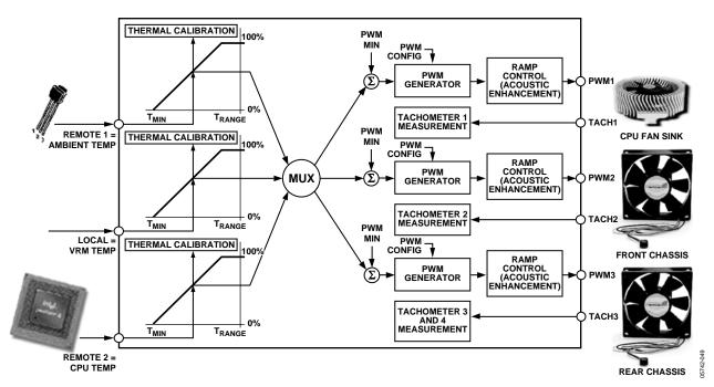
Figure 48. Hardware Configuration Example
