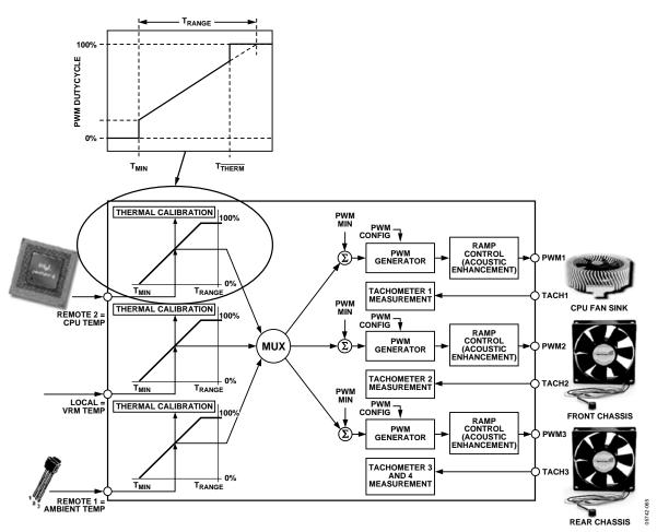
Figure 64. How T<sub>THERM</sub> Relates to Automatic Fan Control
