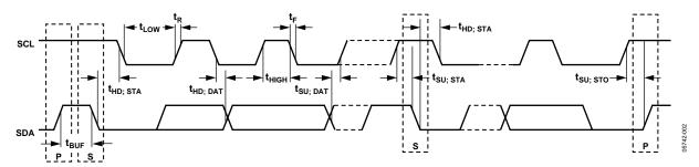
Figure 2. Serial Bus Timing Diagram
