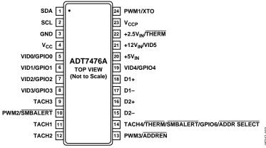
Figure 3. Pin Configuration
