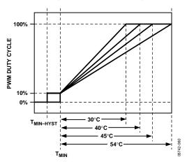
Figure 59. Increasing T<sub>RANGE</sub> Changes the AFC slope
