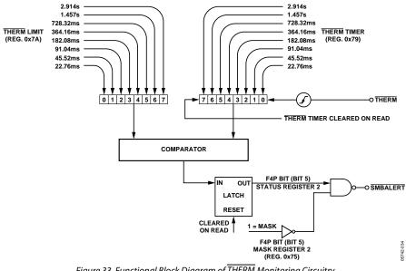
Figure 33. Functional Block Diagram of THERM Monitoring Circuitry
