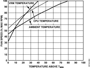
Figure 63. T<sub>RANGE</sub> and % Fan Speed Slopes for VRM, Ambient, and CPU Temperature Channels
