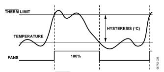
Figure 28. THERM Temperature Limit Operation
