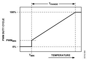
Figure 57. T<sub>RANGE</sub> Parameter Affects Cooling Slope
