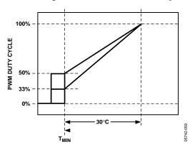
Figure 58. Adjusting PWM<sub>MIN</sub> Changes the Automatic Fan Control Slope.
