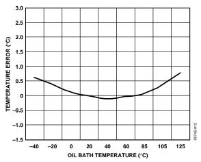
Figure 11. Internal Temperature Error vs. ADT7476A Temperature
