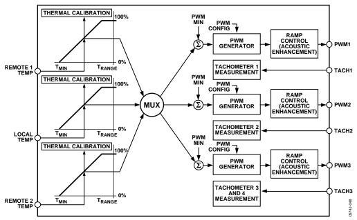
Figure 47. Automatic Fan Control Block Diagram
