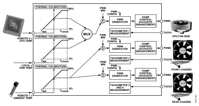
Figure 52. Mux Configuration Example
