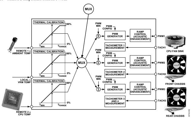
Figure 51. Assigning Temperature Channels to Fan Channels
