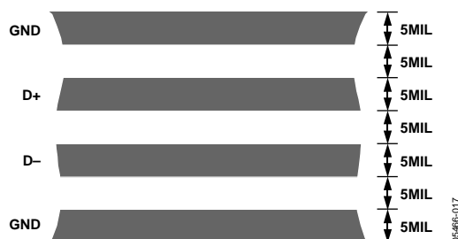
Figure 22. Typical Arrangement of Signal Tracks
