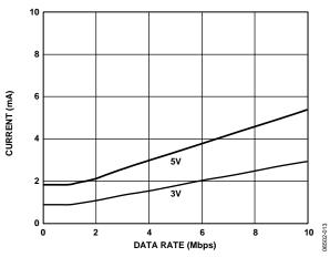
Figure 13. Typical ADuM1411 V<sub>DD1</sub> Supply Current vs. Data Rate for 5 V and 3 V Operation
