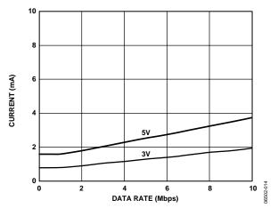
Figure 14. Typical ADuM1411 V<sub>DD2</sub> Supply Current vs. Data Rate for 5 V and 3 V Operation
