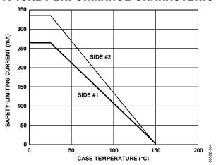
Figure 7. Thermal Derating Curve, Dependence of Safety-Limiting Values with Case Temperature per DIN EN 60747-5-2
