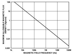
Figure 18. Maximum Allowable External Magnetic Flux Density
