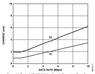
Figure 11. Typical ADuM1410 V<sub>DD1</sub> Supply Current vs. Data Rate for 5 V and 3 V Operation
