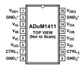
\*PIN 2 AND PIN 8 ARE INTERNALLY CONNECTED. CONNECTING BOTH TO  $\mathrm{GND_1}$  IS RECOMMENDED. PIN 9 AND PIN 15 ARE INTERNALLY CONNECTED. CONNECTING BOTH TO  $\mathrm{GND_2}$  IS RECOMMENDED.
