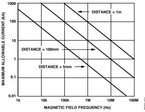
Figure 7. Maximum Allowable Current for Various Current-to-ADuM6132 Spacings
