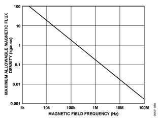
Figure 6. Maximum Allowable External Magnetic Flux Density
