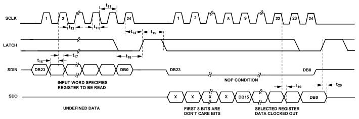
Figure 3. Readback Mode Timing Diagram
