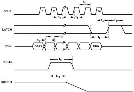
Figure 2. Write Mode Timing Diagram
