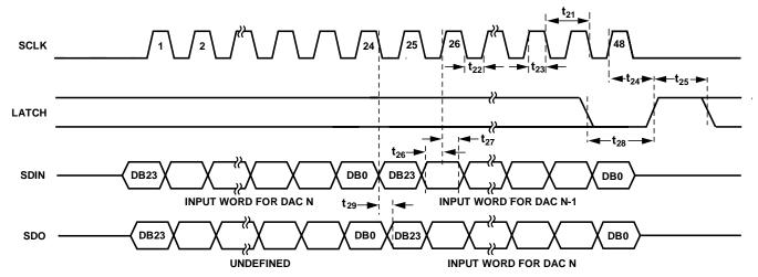
Figure 4. Daisychain Mode Timing Diagram
