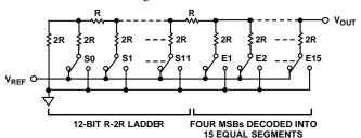
Figure 57. DAC Ladder Structure
