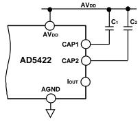
Figure 62. IOUT Filtering Capacitors
