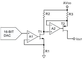
Figure 58. Voltage to Current conversion circuitry
