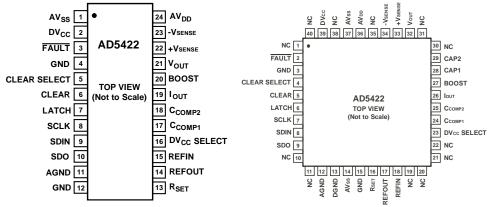
Figure 5. TSSOP Pin Configuration
