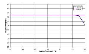
Figure 66. Maximum Supply Voltage Vs Ambient Temperature
