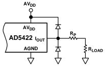
Figure 63. Output Transient Voltage Protection
