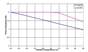
Figure 65. Maximum Power Dissipation Vs Ambient Temperature
