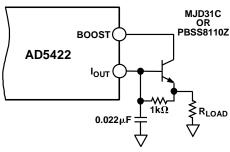
Figure 61. External Boost Configuration
