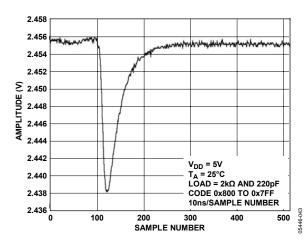
Figure 32. Digital-to-Analog Glitch Impulse
