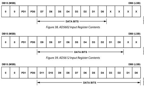
Figure 40. AD5622 Input Register Contents
