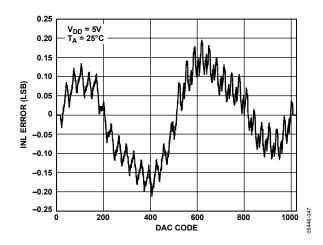
Figure 6. Typical AD5612 Integral Nonlinearity Error
