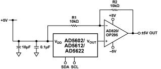
Figure 50. Bipolar Operation with the AD5602/AD5612/AD5622
