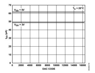
Figure 23. Supply Current vs. Digital Input Code
