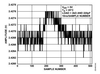
Figure 33. Digital Feedthrough
