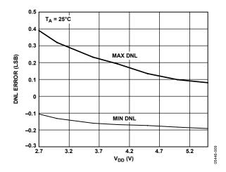
Figure 13. AD5622 DNL Error vs. Supply
