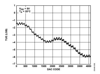
Figure 10. Typical AD5622 Total Unadjusted Error
