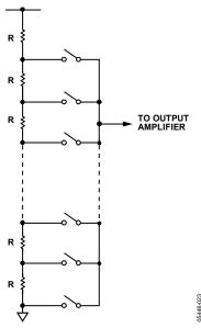
Figure 37. Resistor String Structure
