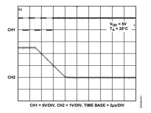
Figure 30. Half-Scale Settling Time
