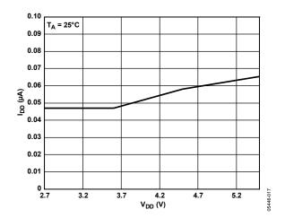
Figure 21. Supply Current vs. Supply Voltage
