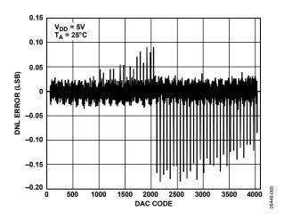
Figure 5. Typical AD5622 Differential Nonlinearity Error
