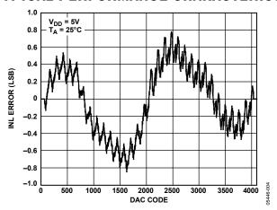
Figure 4. Typical AD5622 Integral Nonlinearity Error
