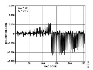
Figure 9. Typical AD5602 Differential Nonlinearity Error
