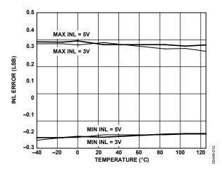
Figure 14. AD5622 INL Error vs. Temperature (3 V/5 V Supply)
