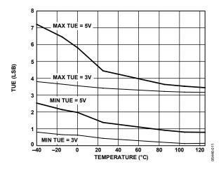
Figure 15. AD5622 Total Unadjusted Error vs. Temperature (3 V/5 V Supply)
