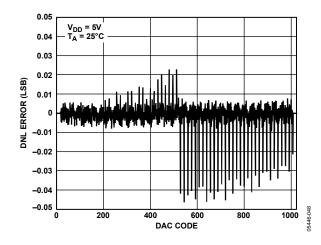
Figure 7. Typical AD5612 Differential Nonlinearity Error
