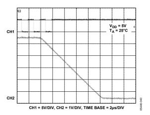
Figure 29. Full-Scale Settling Time
