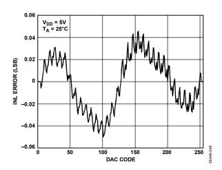
Figure 8. Typical AD5602 Integral Nonlinearity Error
