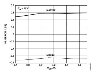
Figure 11. AD5622 INL Error vs. Supply
