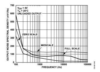
Figure 35. Output Noise Spectral Density
