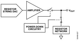
Figure 41. Output Stage During Power-Down
