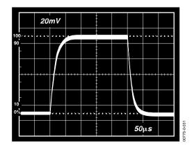
Figure 31. Small Signal Pulse Response, G = 1000,  $R_L$  = 2 k $\Omega$ ,  $C_L$  = 100 pF
