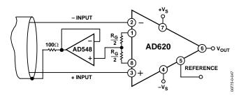
Figure 45. Common-Mode Shield Driver
