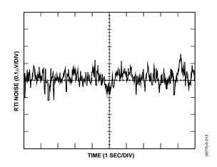
Figure 13. 0.1 Hz to 10 Hz RTI Voltage Noise (G = 1000)
