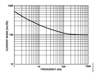
Figure 11. Current Noise Spectral Density vs. Frequency
