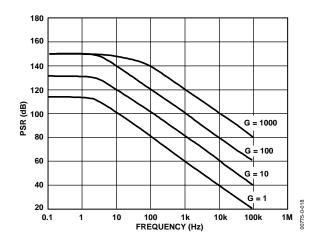
Figure 18. Negative PSR vs. Frequency, RTI (G = 1-1000)
