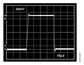
Figure 27. Small Signal Response, G = 10,  $R_L = 2 k\Omega$ ,  $C_L = 100 pF$
