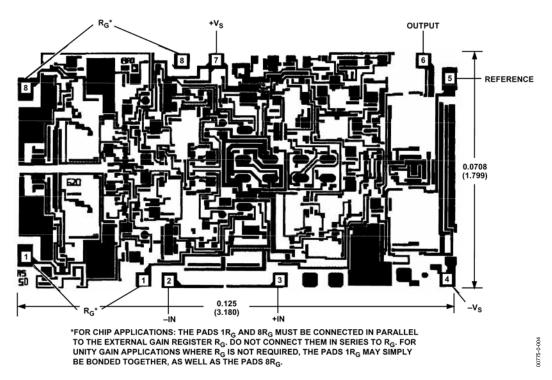
Figure 4. Metallization Photograph. Dimensions shown in inches and (mm).
