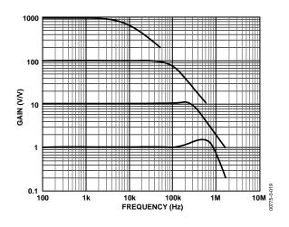
Figure 19. Gain vs. Frequency
