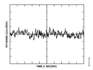
Figure 12. 0.1 Hz to 10 Hz RTI Voltage Noise (G = 1)
