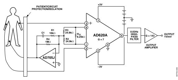
Figure 41. A Medical ECG Monitor Circuit
