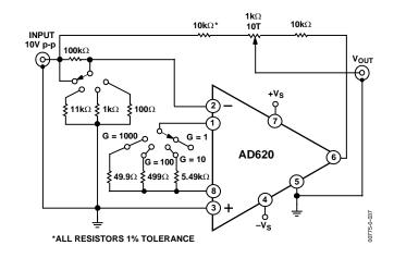
Figure 37. Settling Time Test Circuit
