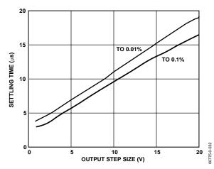
Figure 32. Settling Time vs. Step Size (G = 1)
