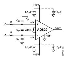
Figure 43. Circuit to Attenuate RF Interference
