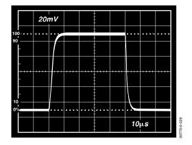
Figure 29. Small Signal Pulse Response, G = 100,  $R_L = 2 k\Omega$ ,  $C_L = 100 pF$
