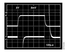
Figure 30. Large Signal Response and Settling Time, G = 1000 (0.5 mV = 0.01%)
