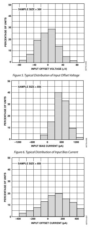
Figure 7. Typical Distribution of Input Offset Current
