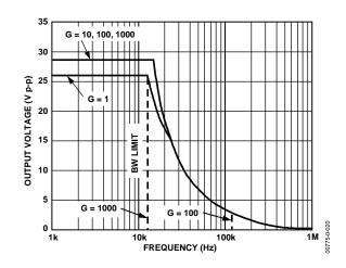
Figure 20. Large Signal Frequency Response
