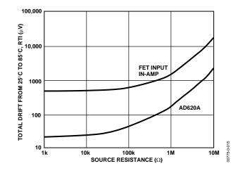
Figure 15. Total Drift vs. Source Resistance
