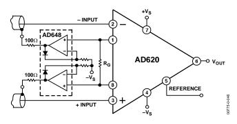
Figure 44. Differential Shield Driver
