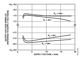
Figure 22. Output Voltage Swing vs. Supply Voltage, G = 10
