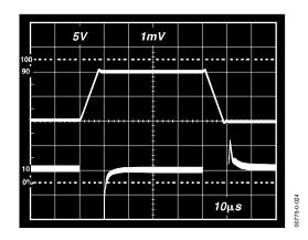
Figure 24. Large Signal Pulse Response and Settling Time G = 1 (0.5 mV = 0.01%)
