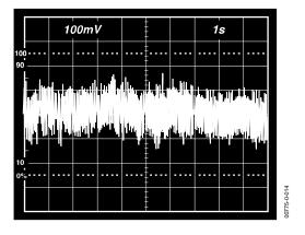
Figure 14. 0.1 Hz to 10 Hz Current Noise, 5 pA/Div
