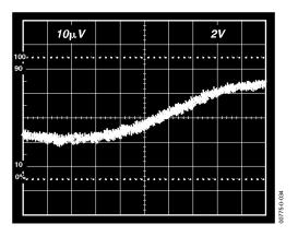
*Figure 34. Gain Nonlinearity,* G = 1,  $R_L = 10 k\Omega (10 \mu V = 1 ppm)$
