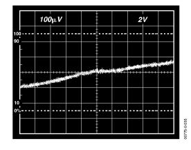
Figure 35. Gain Nonlinearity, G = 100, R<sub>L</sub> = 10 k $\Omega$  (100  $\mu V$  = 10 ppm)
