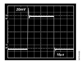
Figure 25. Small Signal Response, G = 1,  $R_L = 2 k\Omega$ ,  $C_L = 100 pF$
