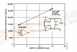
Figure 2. Three Op Amp IA Designs vs. AD620
