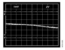
Figure 36. Gain Nonlinearity, G = 1000, R\_L = 10 k\Omega (1 mV = 100 ppm)
