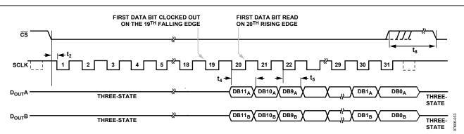
Figure 33. Serial Interface Timing Diagram When Reading Data on the 20th Rising SCLK Edge with a 40 MHz SCLK
