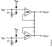
Figure 24. Analog Input Structure
