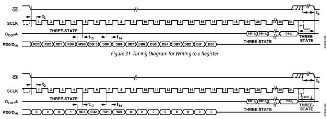
Figure 32. Timing Diagram for a Read Operation with PD0/D<sub>IN</sub> as an Input
