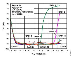
Figure 19. THD vs. Common-Mode Range for Various PGA Gain Settings
