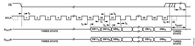
Figure 2. Serial Interface Timing Diagram
