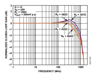
Figure 6. Small Signal Feedback Resistor (R<sub>F</sub>) Optimization
