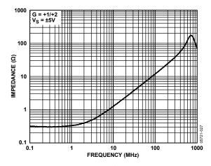
Figure 26. Output Impedance vs. Frequency
