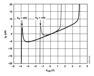
Figure 31. Noninverting Input Bias Current vs. Common-Mode Range
