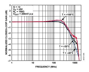
Figure 8. Small Signal Frequency Response for Various Temperatures
