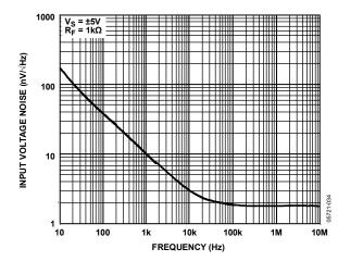
Figure 34. Input Voltage Noise vs. Frequency
