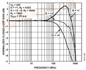
Figure 2. Large Signal Frequency Response for Various Gains
