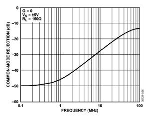
Figure 24. Common-Mode Rejection vs. Frequency
