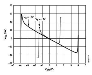
Figure 28. Offset Voltage vs. Input Common-Mode Range
