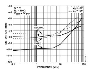
Figure 12. Harmonic Distortion vs. Frequency for Various Supplies
