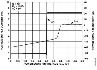
Figure 33. POWER DOWN Pin Current and Supply Current vs. POWER DOWN Pin Voltage
