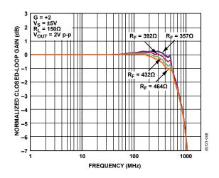
Figure 9. Large Signal Feedback Resistor (R<sub>F</sub>) Optimization
