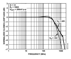
Figure 5. Small Signal Frequency Response for Various Supplies
