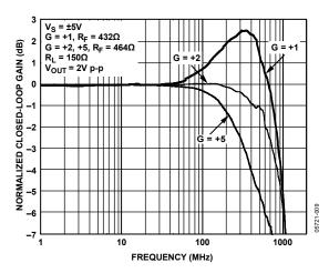
Figure 11. Large Signal Frequency Response for Various Gains
