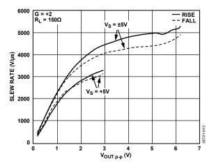
Figure 22. Slew Rate vs. Output Voltage
