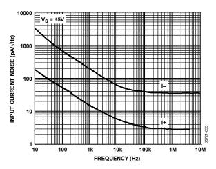
Figure 36. Input Current Noise vs. Frequency
