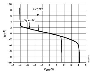
Figure 29. Inverting Input Bias Current Linearity
