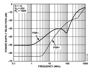
Figure 27. Power Supply Rejection vs. Frequency
