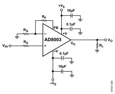
Figure 38. Noninverting Gain
