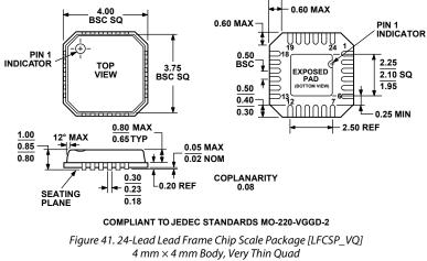
4 mm × 4 mm Body, Very Thin Quad (CP-24-1) Dimensions shown in millimeters
