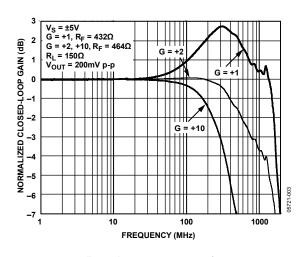
Figure 7. Small Signal Frequency Response for Various Gains
