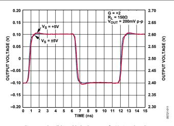
Figure 19. Small Signal Pulse Response for Various Supplies
