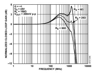
Figure 10. G = +1 Series Resistor (R<sub>5</sub>) Optimization
