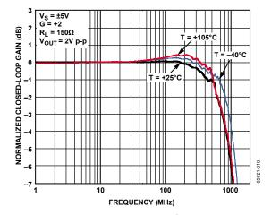
Figure 14. Large Signal Frequency Response for Various Temperatures
