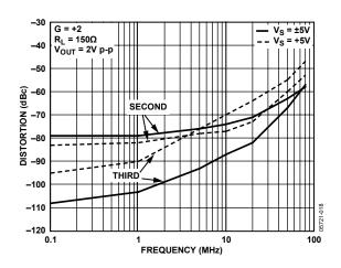
Figure 15. Harmonic Distortion vs. Frequency for Various Supplies
