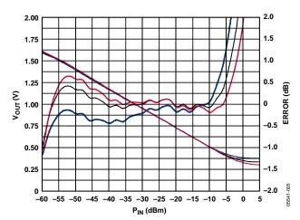
Figure 5.  $V_{\text{OUT}}$  and Log Conformance vs. Input Amplitude at 2.2 GHz,  $R_{\text{TADJ}} = 8 \text{ k}\Omega$
