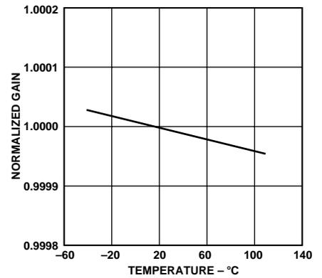
Figure 9. Normalized Gain vs. Temperature,  $G = 1$
