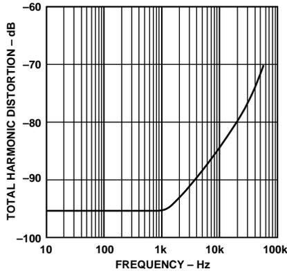
Figure 23. Total Harmonic Distortion vs. Frequency Gain = 16
