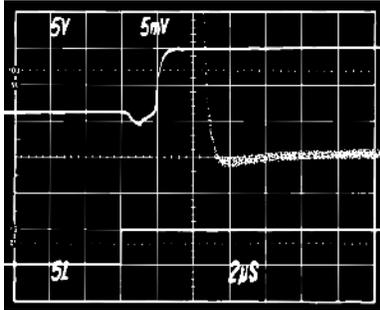
Figure 28. Gain Change Settling Time,\* Gain Change 1 to 8
