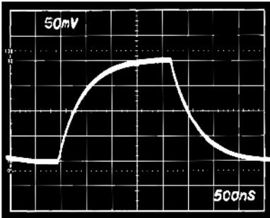
Figure 22. Small Signal Pulse Response, Gain = 16
