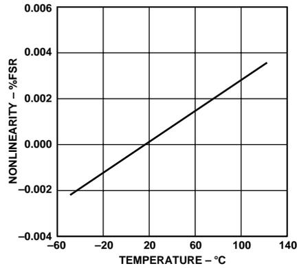
Figure 11. Nonlinearity vs. Temperature, Gain = 1
