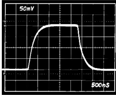
Figure 20. Small Signal Pulse Response, G = 8
