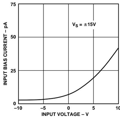
Figure 5. Input Bias Current vs. Input Voltage
