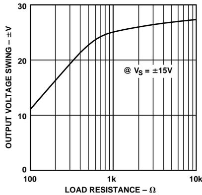
Figure 2. Output Voltage Swing vs. Load Resistance
