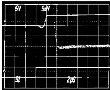
Figure 26. Gain Change Settling Time,\*\* Gain Change: 1 to 2
