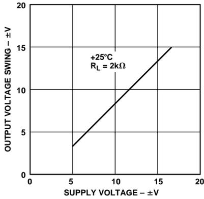
Figure 1. Output Voltage Swing vs. Supply Voltage,  $G = 16$
