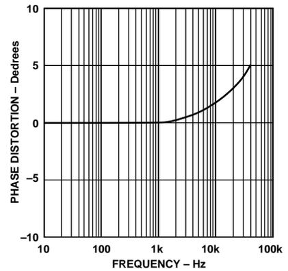
Figure 24. Phase Distortion vs. Frequency, Gain = 16
