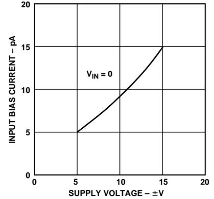
Figure 3. Input Bias Current vs. Supply Voltage
