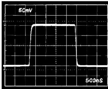
Figure 14. Small Signal Pulse Response, G = 1
