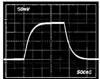
Figure 18. Small Signal Pulse Response, G = 4
