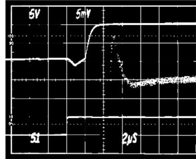
Figure 29. Gain Change Settling Time,\* Gain Change 1 to 16
