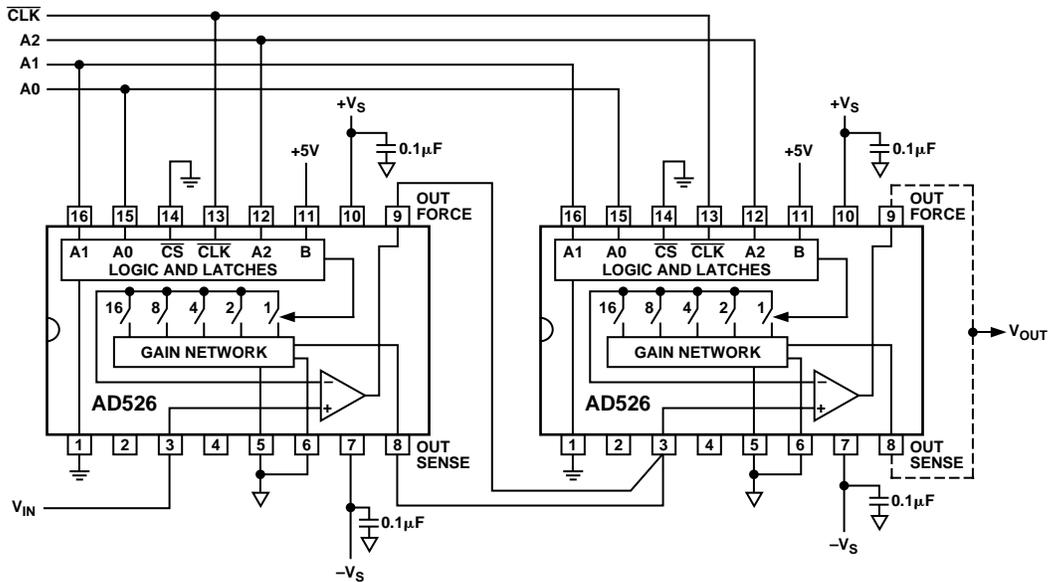
Figure 38. Cascaded Operation
