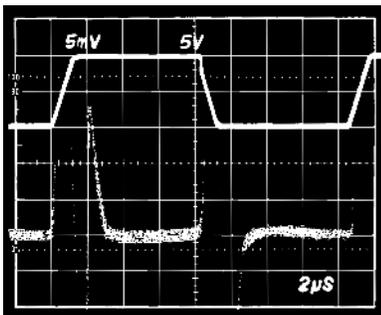
Figure 16. Small Signal Pulse Response, G = 2
