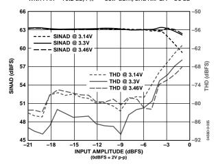
Figure 5. SINAD and THD vs. Input Amplitude and Supply  $(f_{IN} = 8 \text{ MHz}, \text{LPF } f_{-3 \text{ dB}} = 26 \text{ MHz}; \text{Rx PGA} = 0 \text{ dB})$
