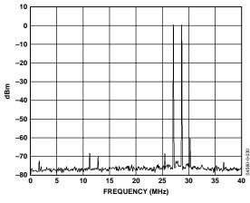
Figure 30. Dual-Tone Spectral Plot of TxDAC's Output ( $f_{DATA} = 80$  MSPS, 2× Interpolation, 10 dBm Peak Power, F1 = 27.1 MHz, F2 = 28.7 MHz)
