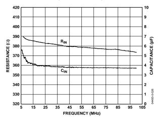
Figure 26. Rx Input Impedance vs. Frequency
