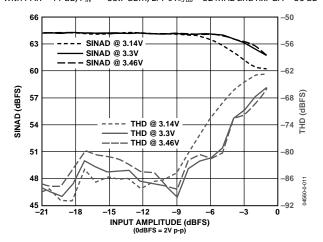
Figure 11. SINAD and THD vs. Input Amplitude and Supply  $(f_{IN}=8\,\text{MHz}, \text{LPF}\,f_{-3\,\text{dB}}=26\,\text{MHz}; \text{RxPGA}=0\,\text{dB})$
