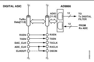
Figure 51. Example of a Half-Duplex Digital Interface with AD9866 Serving as the Slave
