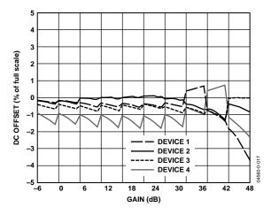
Figure 17. Rx DC Offset vs. RxPGA Gain
