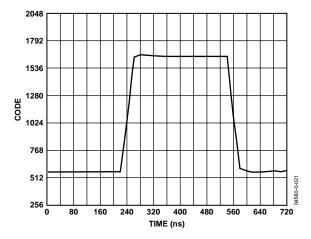
Figure 21. RxPGA Settling Time -12 dB to +48 dB Transition for DC Input  $(f_{ADC} = 50 \text{ MSPS}, \text{LPF Disabled})$
