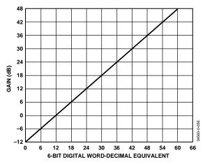
Figure 56. Digital Gain Mapping of RxPGA
