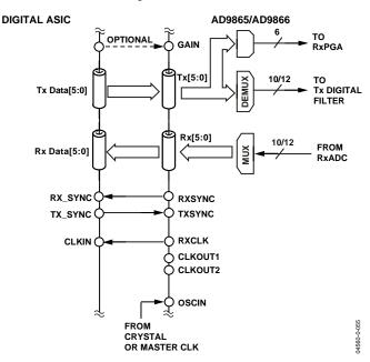
Figure 55. Example of a Full-Duplex Digital Interface with Optional RxPGA Gain Control via Tx[5:0]
