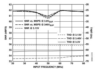
Figure 18. SNR and THD vs. Sample Rate and Supply (LPF Disabled; RxPGA = 0 dB;  $f_{\rm IN}$  = 8 MHz)
