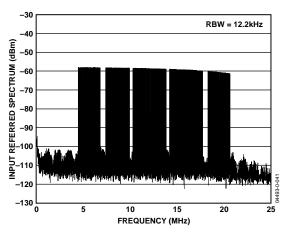
Figure 4. Spectral Plot with 4k FFT of 84-Carrier DMT Signal with PAR = 10.2 dB,  $P_{IN} = -33.7 \text{ dBm}$ , and RxPGA = 36 dB
