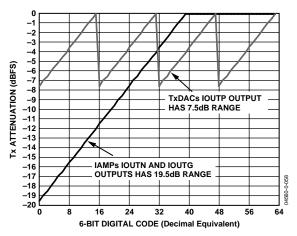
Figure 58. Digital Gain Mapping of TxPGA
