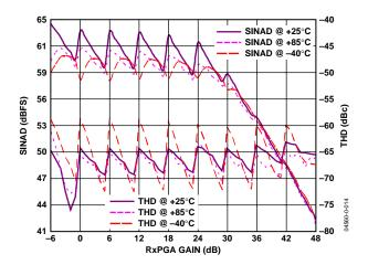
Figure 14. SINAD/THD Performance vs. RxPGA Gain and Temperature (  $f_{\rm IN}$  = 10 MHz)
