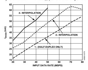
Figure 79. Digital Supply Current Consumption vs. Input Data Rate  $(DVDD = DRVDD = 3.3 V \text{ and } f_{OUT} = f_{DATA}/10)$
