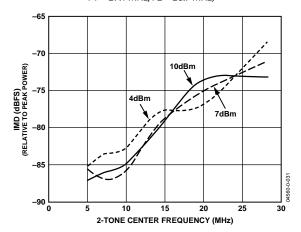
Figure 31. 2-Tone IMD Frequency Sweep vs. Peak Power with f<sub>DATA</sub> = 80 MSPS, 2× Interpolation
