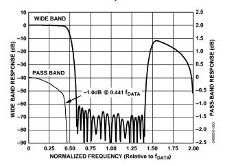
Figure 60. Frequency Response of 2× Interpolation Filter (Normalized to f<sub>DATA</sub>)
