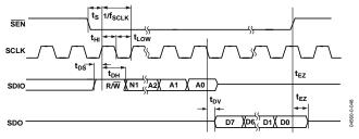
Figure 48. SPI 4-Wire Read Operation Timing
