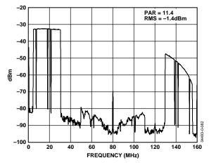
Figure 37. Wideband Spectral Plot of 111-Carrier OFDM Test Vector  $(f_{DATA} = 80 \text{ MSPS}, 2 \times \text{Interpolation})$
