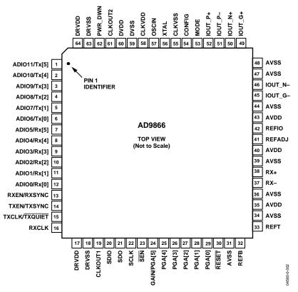
Figure 2. Pin Configuration
