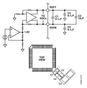
Figure 75. ADC Reference and Decoupling
