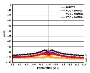
Figure 77. Comparison of Phase Noise Performance when ADC Clock Source is Derived from Different VCO Output Frequencies
