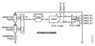
Figure 59. Functional Block Diagram of Tx Path
