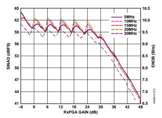
Figure 12. SINAD/ENOB vs. RxPGA Gain and Frequency
