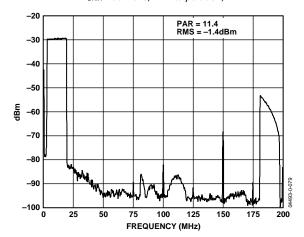
Figure 34. Wideband Spectral Plot of 88-Subcarrier OFDM Test Vector  $(f_{DATA} = 50 \text{ MSPS}, 4 \times \text{Interpolation})$
