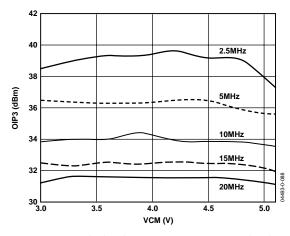
Figure 43. IOUTG Third-Order Intercept vs. Common-Mode Voltage (IAMP Settings of I = 4.25 mA, N = 0, G = 6, 2:1 Transformer into  $75 \Omega$  Load)
