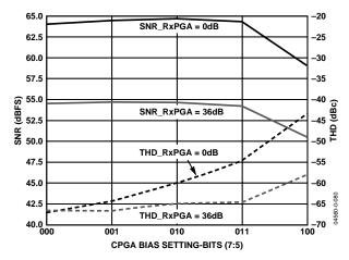
Figure 80. THD vs.  $f_{\rm IN}$  Performance and RxPGA Bias Settings (000,001,010,100 with RxPGA = 0 and +36 dB and AIN = -1 dBFS, LPF set to 26 MHz and  $f_{\rm ADC}$  = 50 MSPS)
