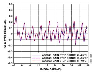
Figure 20. RxPGA Gain Step Error vs. Gain ( $f_{IN} = 10 \text{ MHz}$ )
