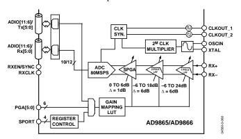
Figure 68. Functional Block Diagram of Rx Path
