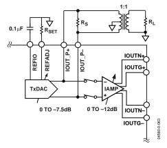
Figure 63. TxDAC Output Directly via Center-Tap Transformer
