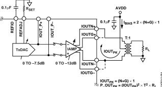
Figure 64. Current-Mode Operation
