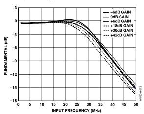
Figure 72. Effects of RxPGA Gain on LPF Frequency Response  $(f_{-3 dB} = 32 \text{ MHz})$  (@ 0 dB and  $f_{ADC} = 80 \text{ MSPS}$ )
