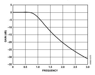
Figure 70. LPF's Normalized Wideband Gain Response
