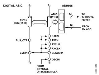
Figure 52. Example of a Half-Duplex Digital Interface with AD9866 Serving as the Master
