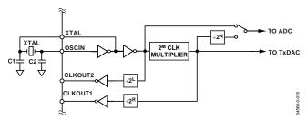
Figure 76. Clock Oscillator and Synthesizer
