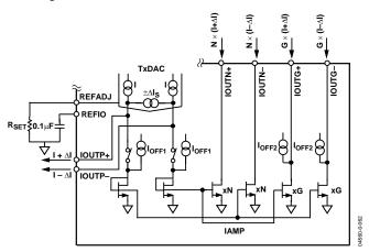
Figure 62. Equivalent Schematic of TxDAC and IAMP
