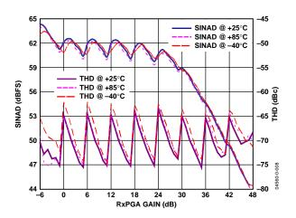
Figure 8. SINAD/THD Performance vs. RxPGA Gain and Temperature ( $f_{IN} = 5 \text{ MHz}$ )
