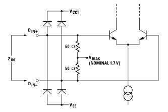
Figure 10. Rx data output equivalent circuit.
