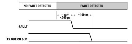
Figure 13. Transmitter FAULT signal timing diagram.
