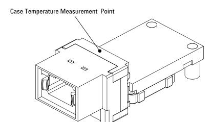
Figure 3. Case temperature measurement. (label and heatsink removed for clarity)
