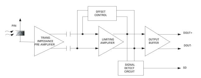
Figure 2. Receiver block diagram (each channel).
