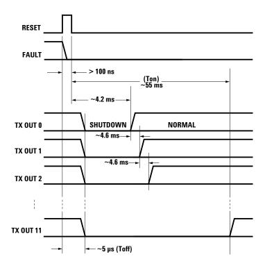
Figure 14. Transmitter RESET timing diagram.
