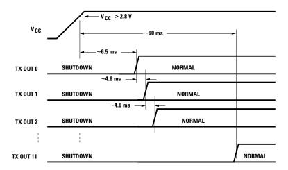
Figure 12. Typical transmitter power-up sequence.
