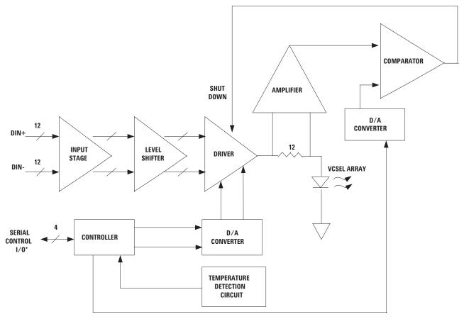
Figure 1. Transmitter block diagram(each channel).  $^*TX\_EN, TX\_DIS, RESET-, FAULT-$
