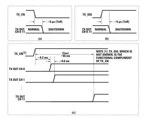
Figure 15. Transmitter TX\_EN and TX\_DIS timing diagram.
