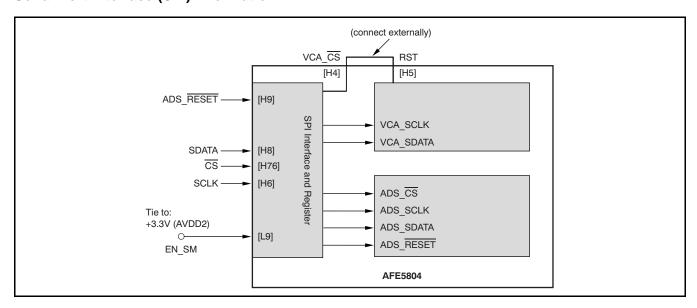
Figure 90. Typical Connection Diagram for the SPI Control Lines
