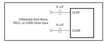
Figure 105. Differential Clock Driving Circuit (DIFF\_CLK = 1)
