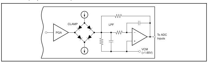
Figure 98. Clamping Stage and Low-Pass Filter (Simplified Schematic)
