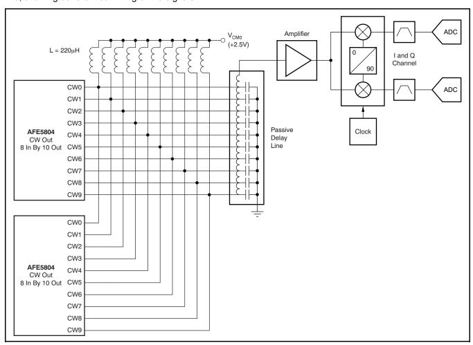
Figure 102. Conceptual CW Doppler Signal Path Using Current Summing and a Passive Delay Line for Beam-Forming
