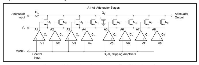
Figure 96. Voltage-Controlled Attenuator Simplified Schematic
