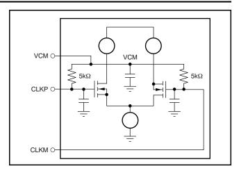
Figure 104. Internal Clock Buffer
