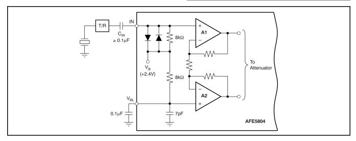
Figure 99. LNA Channel (Simplified Schematic)
