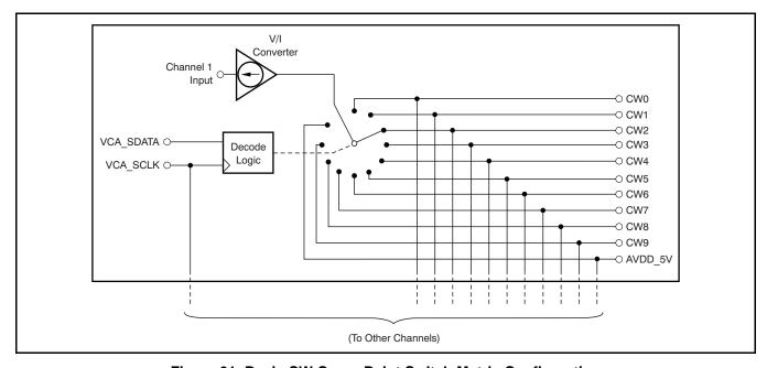
Figure 91. Basic CW Cross-Point Switch Matrix Configuration
