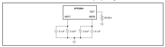
Figure 107. Suggested Decoupling on the Reference Pins
