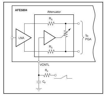
Figure 101. External Filtering of the V<sub>CNTL</sub> Input
