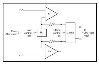
Figure 97. Post-Gain Amplifier (Simplified Schematic)
