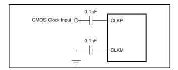
Figure 106. Single-Ended Clock Driving Circuit
