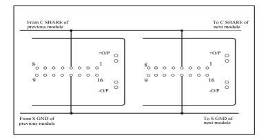
The voltage on the C SHARE pins represents the average load current per module. Each module compares this average with its own current and adjusts its output voltage to correct the error. In this way the module maintains accurate current sharing even under variable or light load conditions.
