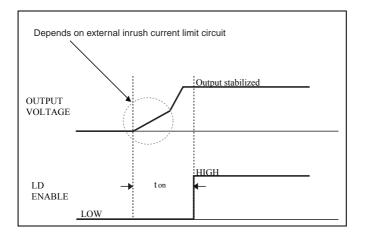
Initially the load is disabled and the LD ENABLE (pin 15) is at 0.4V (LOW). When the PFC power up sequence has completed, the LD ENABLE voltage goes HIGH. And the LD ENABLE will stay high as long as Vin is above 175Vac or Vout is above 250V, even if PF\_ENABLE is in disable mode. (Please see the application example section at P.25 for the external circuit to interlock the LD-ENABLE from PF\_ENABLE)
