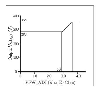
The output from the PFW ADJ pin is a 1mA current source. To adjust the PFW threshold, a voltage source (0 - 4Volts) or a programming resistance (0 - 4Kohm) referenced to s S GND (pin 13) should be connected. This allows adjustment of the PFW threshold from 280V up to 340V. The value of resistance or voltage required can be read from the graph above.
