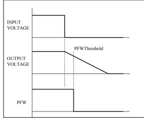
The output of the PFW signal can drive an opto-coupler to provide an isolated signal from primary side to the secondary side. The nominal factory set PFW threshold is set at 340V.
