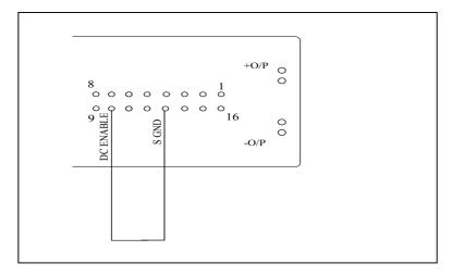
For using DC input, connect the DC ENABLE pin to S GND
