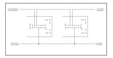
If the clock input to any module fails, the module will automatically switch back to its internal clock and will continue to operate at full power even in current sharing systems. The CLK IN and CLK OUT signals are AC coupled.
