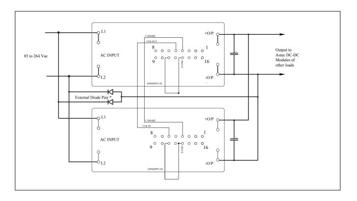
\* The current rate requirement of external rectifier for each line is 20A x number of units in parallel. For example, if there are 3 pieces of AIF04ZPFC-02L in parallel, customer will need to put 60A (20A x 3) external rectifier for each line.
