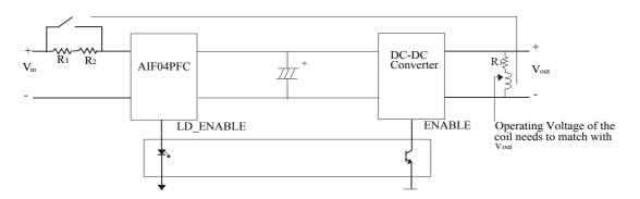
CIRCUIT(2):Using relay controlled by Auxiliary supply on primary side:
