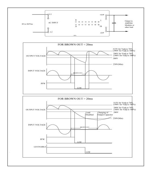
After a Brown Out condition where the output voltage has not dropped below 250Vdc, the module will recover when input power is restored. The PFW signal can be used to monitor input power loss.
