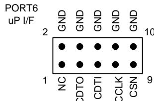
Figure 3. PORT6 pin layout
