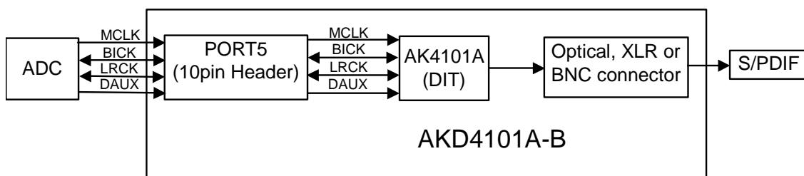
MCLK, BICK, LRCK and DAUX are input via 10pin header (PORT5: DIT). The AKD4101A-B can be connected with the AKM's ADC evaluation board via 10-line cable.
