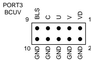
Figure 2. PORT3 pin layout
