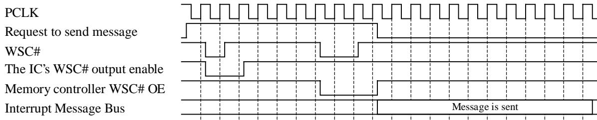
The IC enables WSC# during the PCLK cycle in which it drives WSC# low and the following cycle in which WSC# is driven high. It is expected that the memory controller enables the line for three PCLK cycles. WSC# is required to be driven high for at least one clock before it is allowed to be driven low again.
