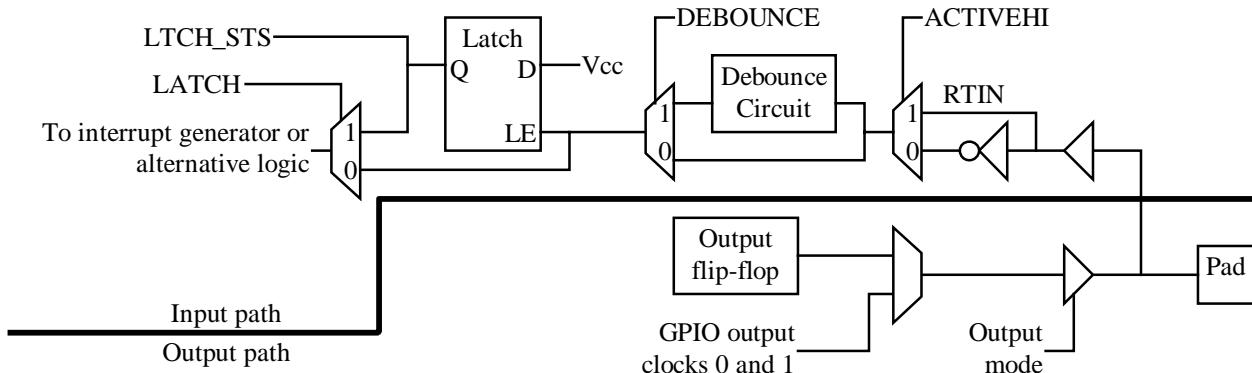
Debounce. The input signal must be active and stable for 12 to 16 milliseconds before the output signal is asserted.
