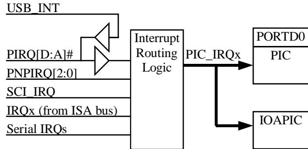
The internal USB interrupt signal drives the PIRQD# pin low as an output; when the USB interrupt is deasserted, PIRQD# is left in the high impedance state. So the USB interrupt is wired-ORed into the active state with external interrupts on PIRQD#. The result enters the IC and goes to the interrupt routing logic.
