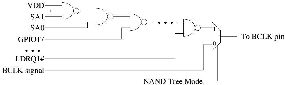
When in NAND tree mode, the five NAND tree output signals are enabled and the remaining signals are in high-impedance mode. The following pins are not part of the NAND tree: RTCX\_IN, RTCX\_OUT, PWRGD, PCLK, TEST#, PGNT#, and SERR#.
