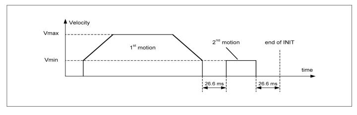
The first motion is done with the specified **Vmin** and **Vmax** velocities in the **RunInit** command, with the acceleration (deceleration) parameter already in RAM, to a position **Pos1[15:0]** also specified in **RunInit**. The goal here is to perform a motion large enough to reach a stall position (considered to be the reference position).
