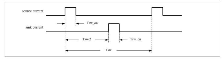
If the switch is detected ON (closed), then the flag <ESW> is raised. The status of this flag can be read by the application via a GetActualPos, a GetStatus or a GetFullstatus reading frame. At the falling edge of every current pulse (at around 1kHz), the stepper-motor actual position is refreshed (register ActPos, see § 9.2.2.9),
