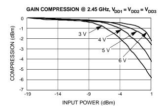
1. All data measured at  $T_A = +25$ °C and  $V_{G1}$ ,  $V_{G2}$  and  $V_{G3}$  adjusted for first stage quiescent current of 20 mA, second stage current of 70 mA and third stage current of 90 mA, respectively.
