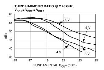
All data measured at T<sub>A</sub> = +25°C and V<sub>G1</sub>, V<sub>G2</sub> and V<sub>G3</sub> adjusted for first stage quiescent current of 20 mA, second stage current of 70 mA and third stage current of 90 mA, respectively.
