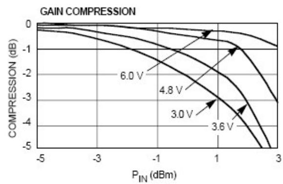
1. All data measured at TA = +25°C and VG1, VG2 adjusted for first stage quiescent current of 30 mA and second stage current of 65 mA, respectively.
