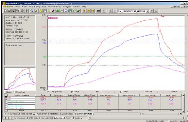
Figure 8: Rework Reflow Profile Rework Profile 1 - Part Removal, Lead-Free Peak temperature: 236.7 °C Time above 217 °C: 82 seconds
