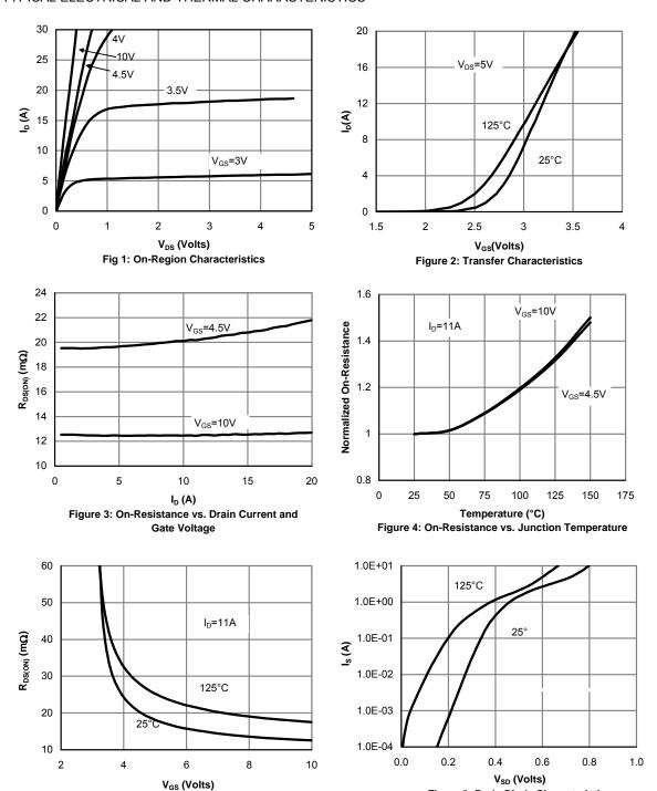
Figure 6: Body-Diode Characteristics
