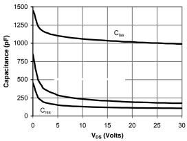
Figure 8: Capacitance Characteristics
