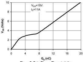
Figure 7: Gate-Charge Characteristics
