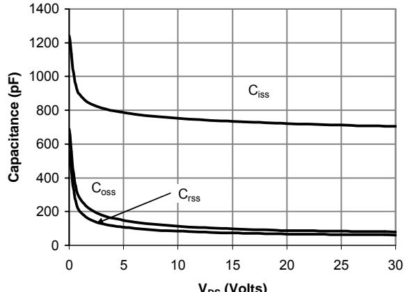
Figure 8: Capacitance Characteristics
