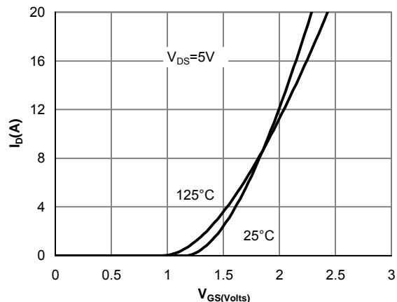
Figure 2: Transfer Characteristics
