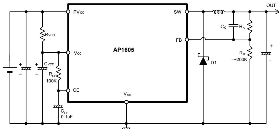
$$V_o = V_{ref} \times \left(1 + \frac{R_A}{R_B}\right)$$
