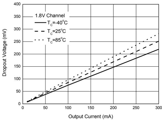
Figure 22. Dropout Voltage vs. Output Current
