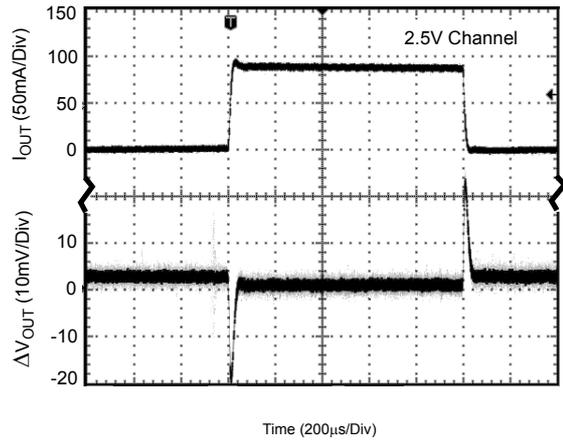
Figure 37. Load Transient
