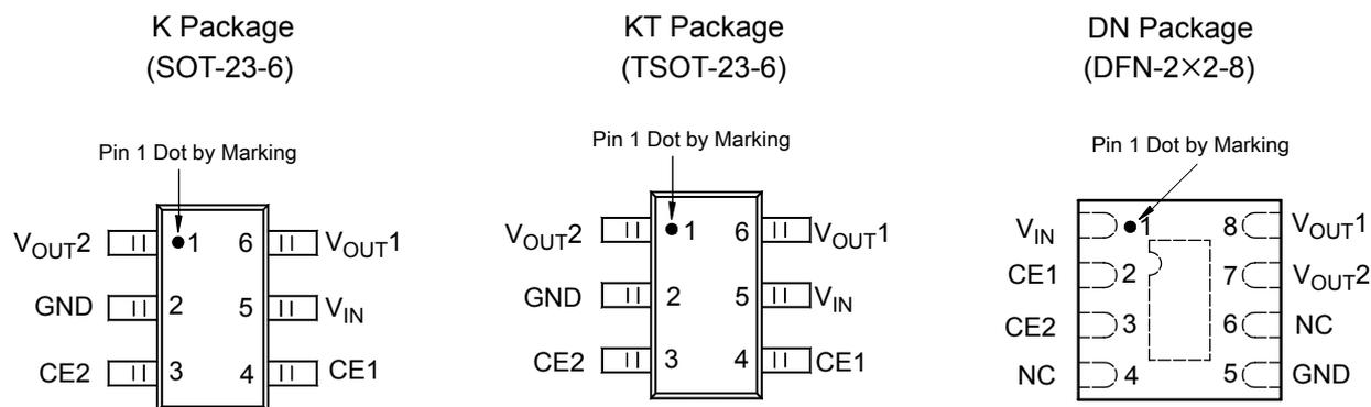
Figure 2. Pin Configuration of AP2402 (Top View)
