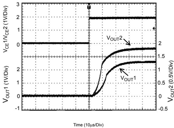
Figure 40. Enable Voltage vs. Output Voltage
