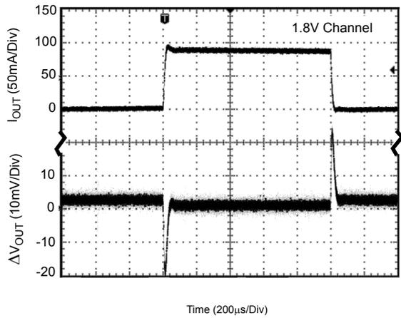
Figure 36. Load Transient
