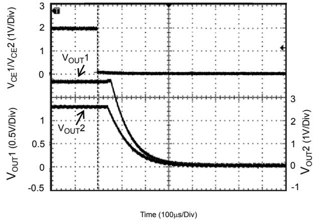
Figure 41. Auto Discharge Function
