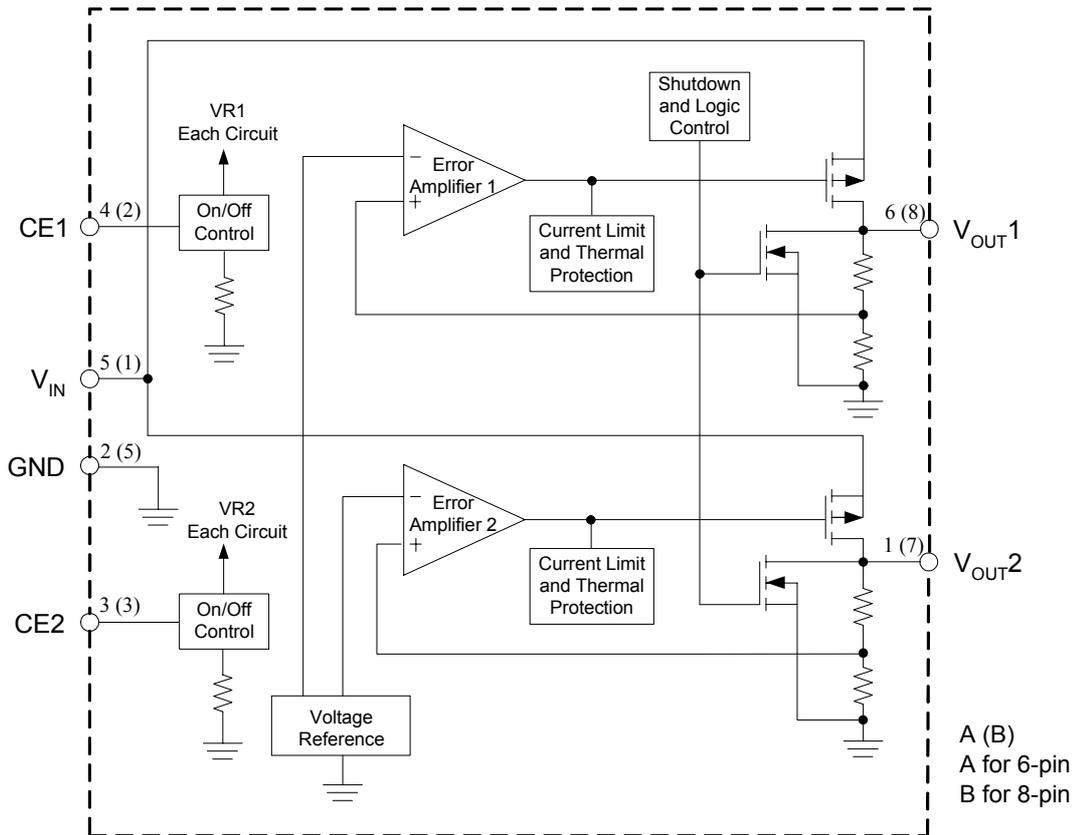
Figure 3. Functional Block Diagram of AP2402
