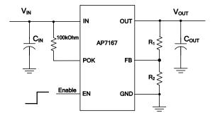
The output voltage is calculated by:
