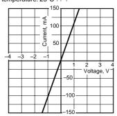
9. Off state leakage current
