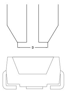
Note: Diameter "D" should be smaller than 2.2mm
