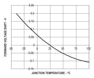
Figure 7. Forward Voltage Shift Vs. Temperature.
