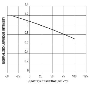
Figure 5. Relative Intensity Vs. Temperature
