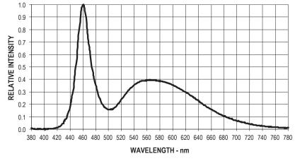
Figure 2. Relative Intensity Vs. Wavelength
