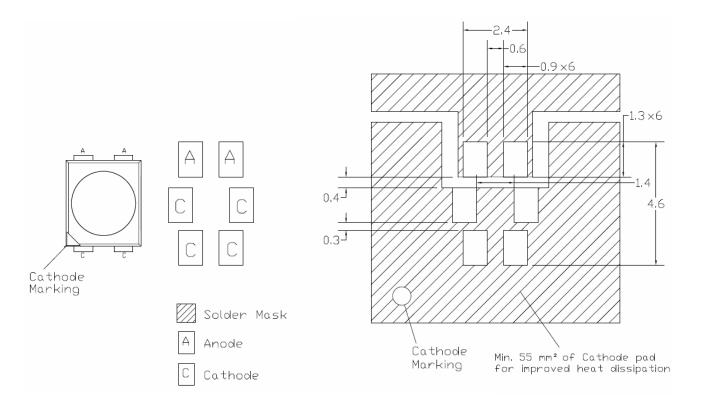
Figure 11. Recommended Soldering Pad Pattern.
