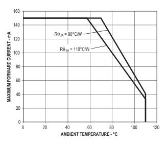
Figure 6a. Maximum Forward Current Vs. Ambient Temperature. Derated Based on  $T_{JMAX}=125\,^{\circ}C,\,R\theta_{J-A}=90\,^{\circ}C/W$  and  $110\,^{\circ}C/W.$
