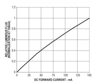
Figure 4. Relative Flux vs. Forward Current
