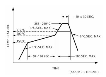
Figure 10. Recommended Pb-free Reflow Soldering Profile.
