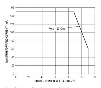
Figure 6b. Maximum forward current vs. solder point temperature. Derated Based on  $T_{JMAX}=125^{\circ}C$  ,  $R\theta_{JP}{=}60^{\circ}C/W$
