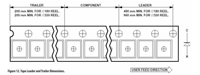
Ø1.5<sup>+0.1</sup> --4 ± 0.1---2 ± 0.05  $-3.6 \pm 0.1$ 1.75 ± 0.1  $\oplus$ 5.5 ± 0.05 3.8 ± 0.1 12<sup>+0.3</sup> -0.1 Ø1+0.1 8 ± 0.1-0.229 ± 0.01 VIEW B-B 3.45 ± 0.1 VIEW A-A ALL DIMENSIONS IN mm.
