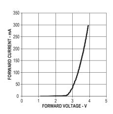
Figure 3. Forward Current Vs. Forward Voltage.
