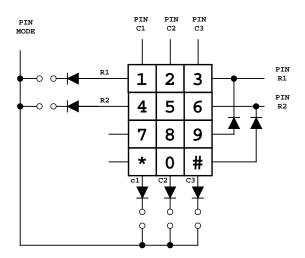
Double contacts under keys 0-9\*#: One contact is connected to AS2540, the other one to CPU.
