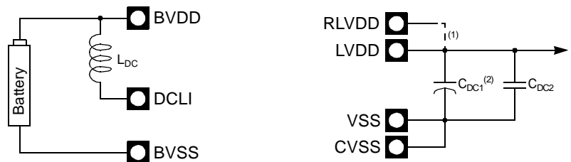
Figure 135. Battery DC-DC Connection
