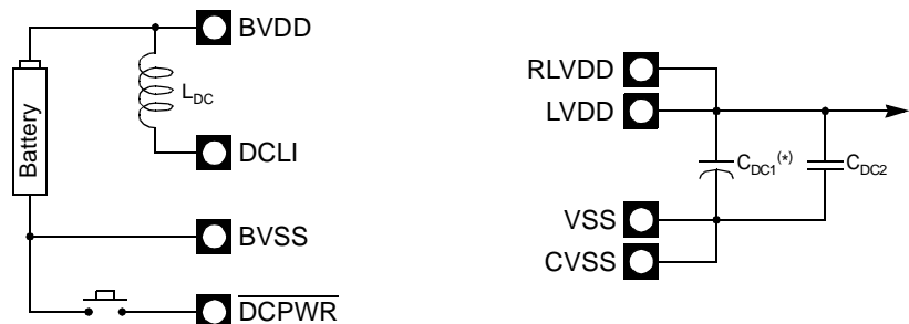
Figure 8. Battery DC-DC Connection
