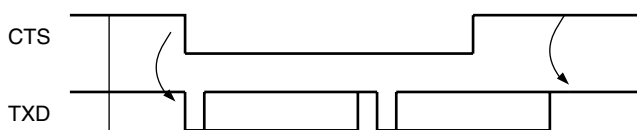
Figure 34-29. Transmitter Behavior when Operating with Hardware Handshaking
