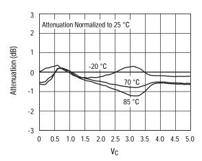
Attenuation vs. Control Voltage Over Temperature
