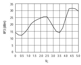
Input IP3 vs. Control Voltage
