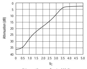
Attenuation vs. Control Voltage
