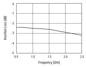
**Insertion Loss vs. Frequency**
