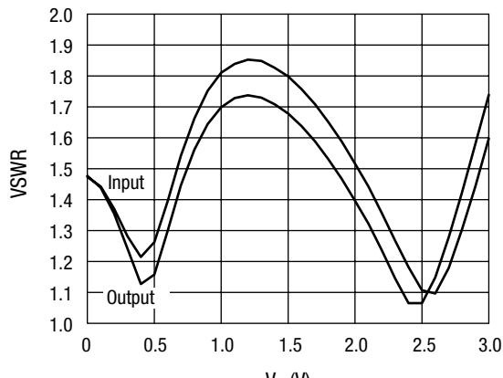
**VSWR vs. Control Voltage**
