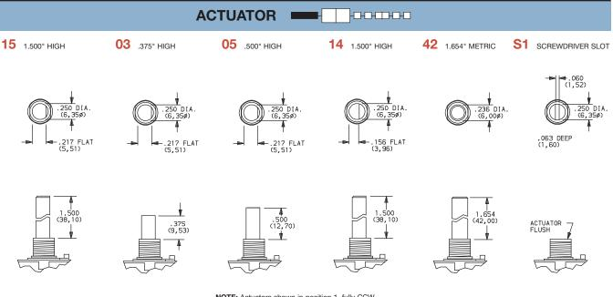
NOTE: Actuators shown in position 1, fully CCW.
