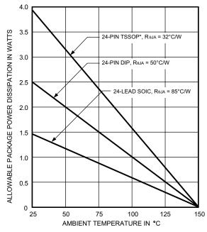
$^*\mbox{Mounted}$  on single-layer, two-sided PCB, with  $3.8~\mbox{in}^2$  copper each side; additional information on Allegro Web site
