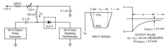
Notes: 1. A 2.0 k $\Omega$  variable resistor adjusted for a Forward Current (I<sub>F</sub>) of 30 mA. 2. Input pulse is adjusted so I<sub>R(peak)</sub> is equal to 30 mA. 3. t<sub>p</sub> » t<sub>rr</sub>
