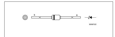
Fig.1 Simplified outline (SOD68; DO-34), pin configuration and symbol.
