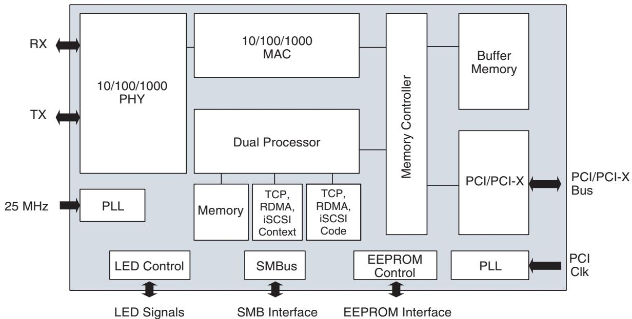
The **BCM5706** provides a fully integrated Layer 4 and Layer 5 solution - TCP/IP, RDMA and iSCSI 1.0/iSER along with a complete 10/100/1000BASE-T Gigabit Ethernet, IEEE 802.3 compliant Media Access Control (MAC) and Physical Layer Transceiver solution for high performance network applications. By itself the **BCM5706** provides a complete single-chip Gigabit Ethernet NIC with a TCP/IP Offload Engine, RDMA NIC (RNIC), iSCSI 1.0/iSER HBA or LOM solution.
