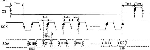
•When CS is "Low", enable micro computer control data (SCK/SDA). (It doesn't work, when it is "High"),
