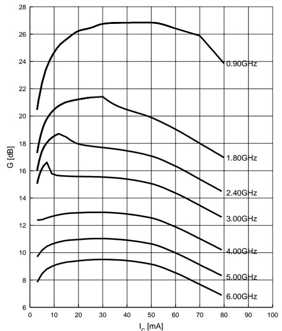
**Power gain  $G_{ma}$ ,  $G_{ms} = f(V_{CE})$**
