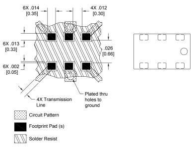
Dimensions are in Inches [Millimeters] Mounting Footprint
