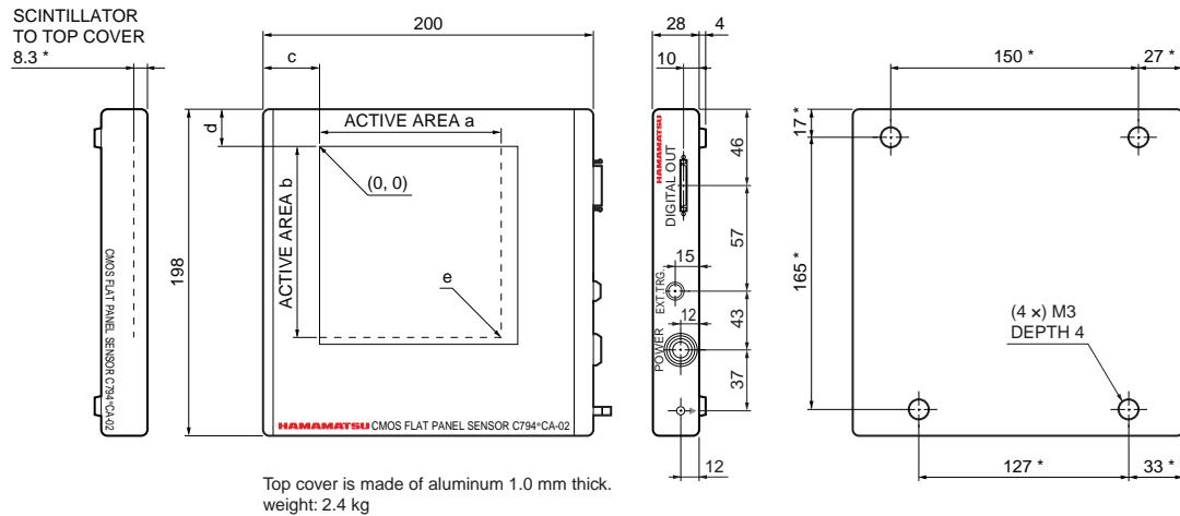
Top cover is made of aluminum 1.0 mm thick.
