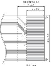
· Mating connectors: FH12-20S-0.5SV vertical type [Made by HIROSE electric] FH12 52745-2090 horizontal type [Made by MOLEX]
