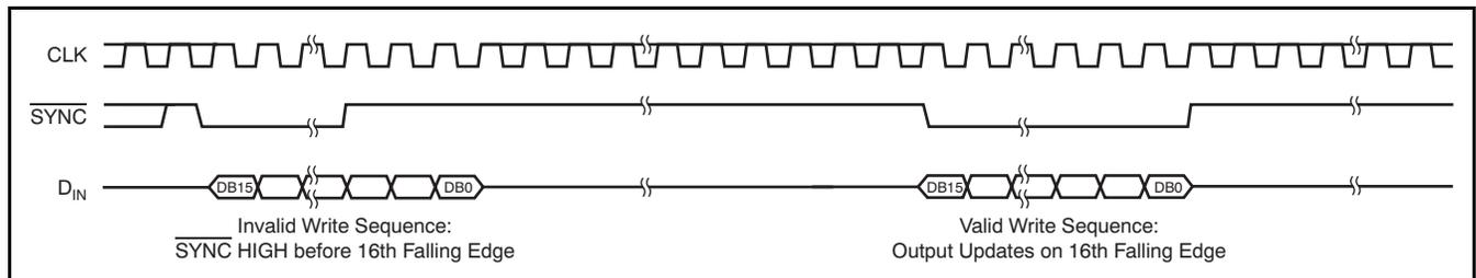
**Figure 112. DACx311  $\overline{\text{SYNC}}$  Interrupt Facility**
