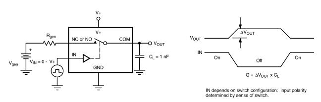
Figure 3. Charge Injection
