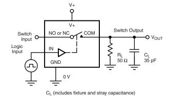
$V_{OUT} = V_{COM} \left( \frac{R_L}{R_L + R_{ON}} \right)$
